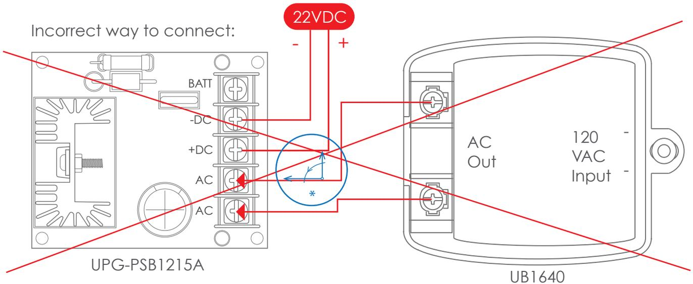
\* Accidentally touching these two wires will cause the output to be 22VDC.
